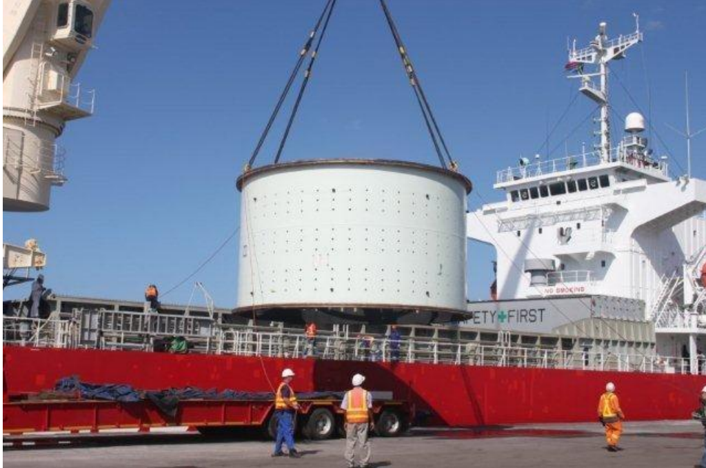
Figure1. Loading SAG mill shell for transport to Australia (which has subsequently arrived in Australia and is ready for transport to site).
