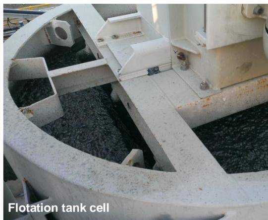
Flotation tank cell
