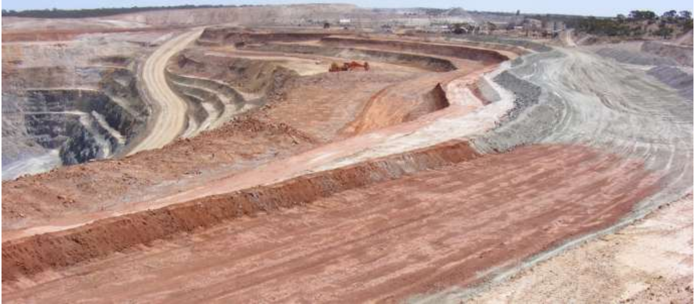
Edna May open pit at 30 September 2013: Stage 1 (base of pit) and Stage 2 (surface)
